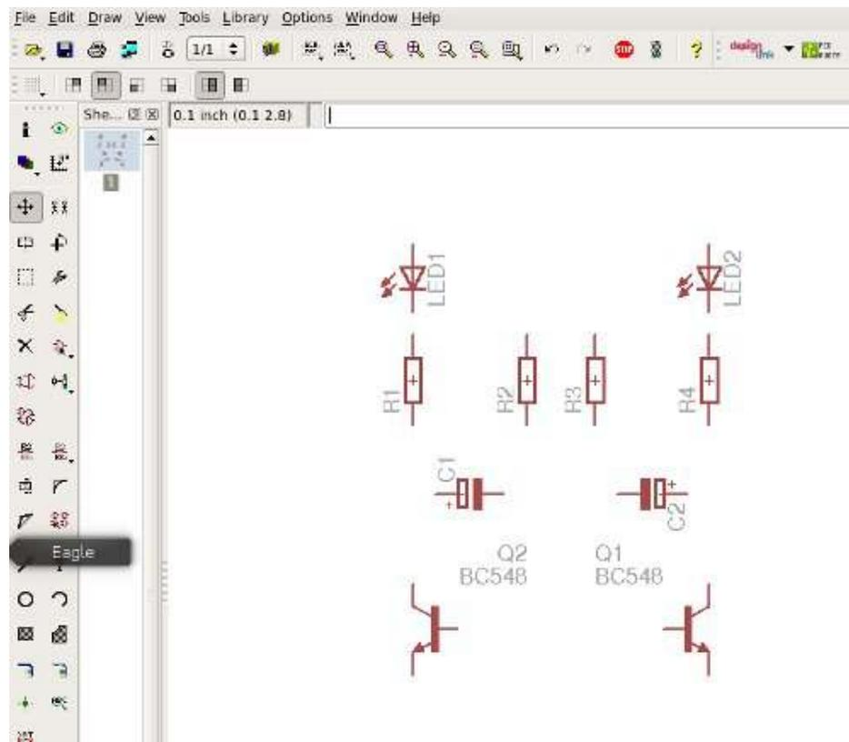
*Tips: To place the two transistor as mirrors to each another like I did, use the Mirror function (**Edit** → **Mirror..**) from the menu.*
