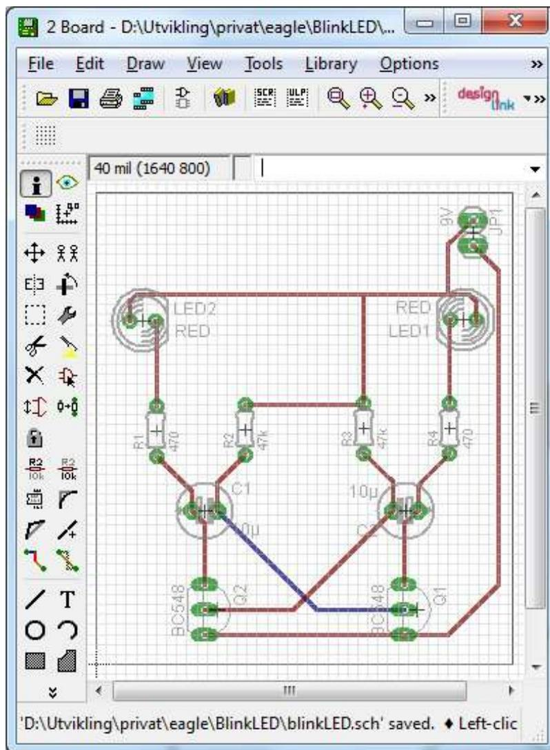
When you have finished routing all the airwires on your board you are ready to prepare the board for manufacturing.
