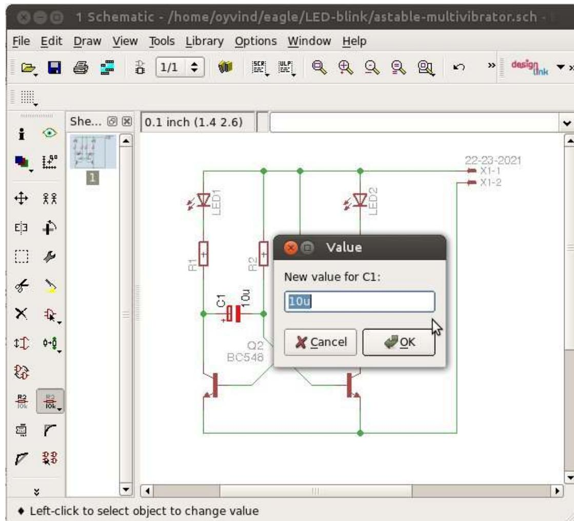
Enter the value and press "Ok". Set values for all the resistors and the capacitors. Use the values from the original drawing of our circuit.
