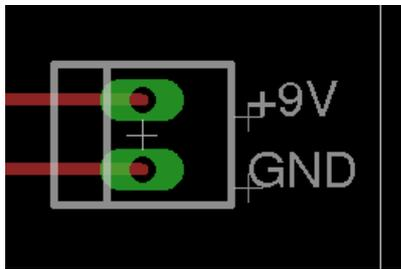
A useful rule-of-thumb is always to label connectors that are going to connect to something outside the board with descriptive names. Add names for each pin on a pin header.
