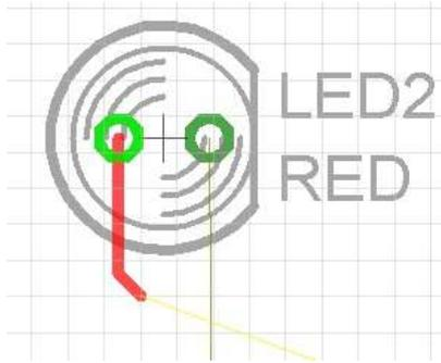
If we want to change the routing layer we simply click the middle mouse button or use the layer selector on the toolbar. If you change routing layer while routing, a via to the next layer is created.
