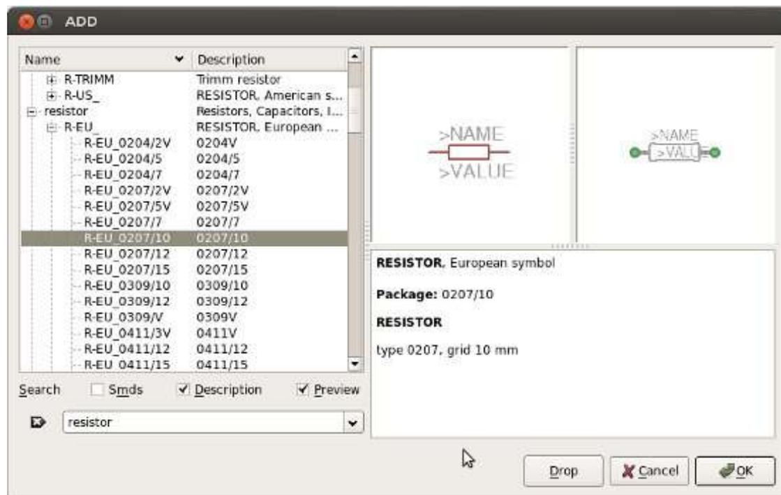
We want to locate a resistor. Write "resistor" in the search field and press Enter. You will probably find many alternatives. I chose a through-hole resistor called R-EU\_0207/10 from the "resistor"-library. Choose one and press "Ok".
