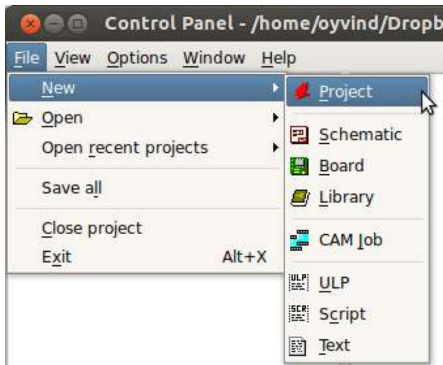
Add a new schematic to the project by selecting **File** → **New** → **Schematic** from the menu. You now have a blank schematic ready for drawing.
