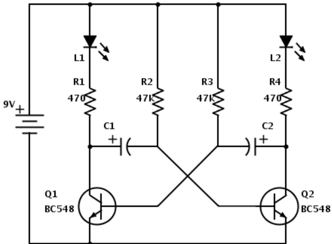
The above schematic is a circuit for making two Light Emitting Diodes (LED) blink. It is called an "Astable Multivibrator". We will use this circuit as an example for the rest of the book.
