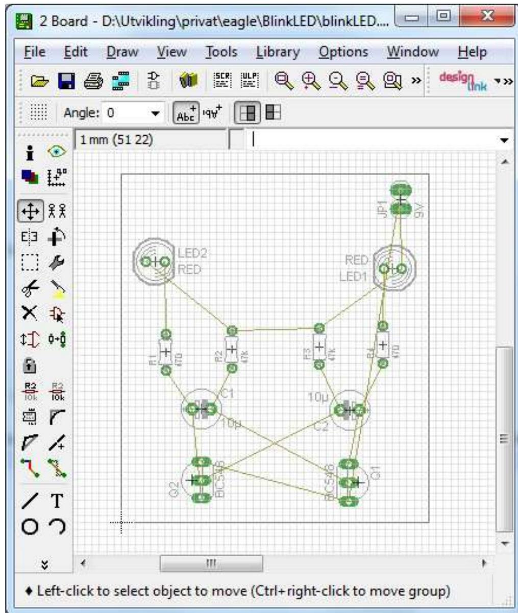
Place all the components within the board limits and arrange them in the same way as the schematic.
