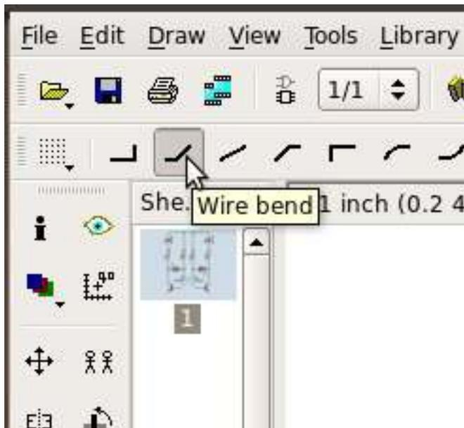
***Tips!*** The "Wire" tool does not always create the electrical connection you want so make it a habit always to use the "Net" tool instead.
