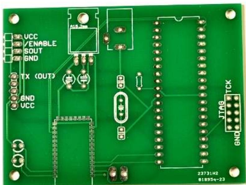
More than one way exists to make a PCB. You can etch boards at home, but I find this messy, unreliable and not worth the effort. You can use a CNC router to create boards, but these machines are usually expensive and vias tend to be much more extra work. Or you can just get your design manufactured by a professional manufacturer for the price of a few bananas. I prefer the latter method ;)
