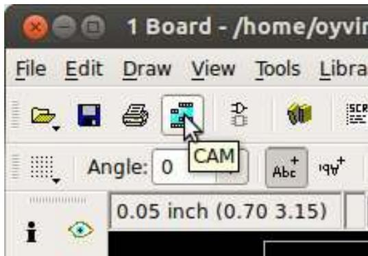
In the board layout window click the "CAM" button or choose **File** → **CAM Processor**. This will open the CAM Processor tool for generating the Gerber files.
